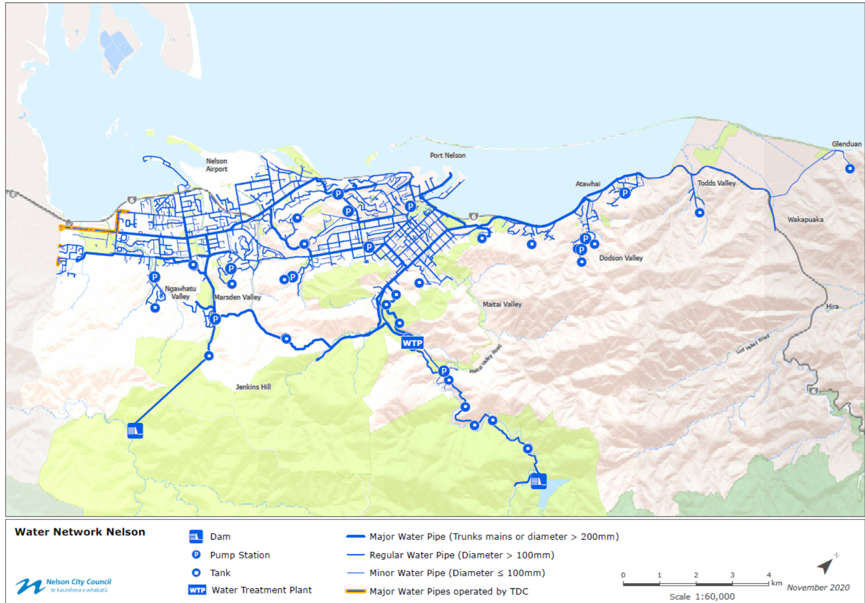
Figure 1-1: Water Network Nelson
