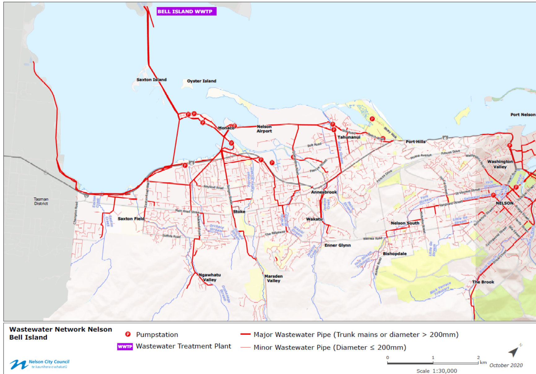
Figure ES-1: Nelson City Wastewater Network Bell Island Wastewater Treatment Plant
