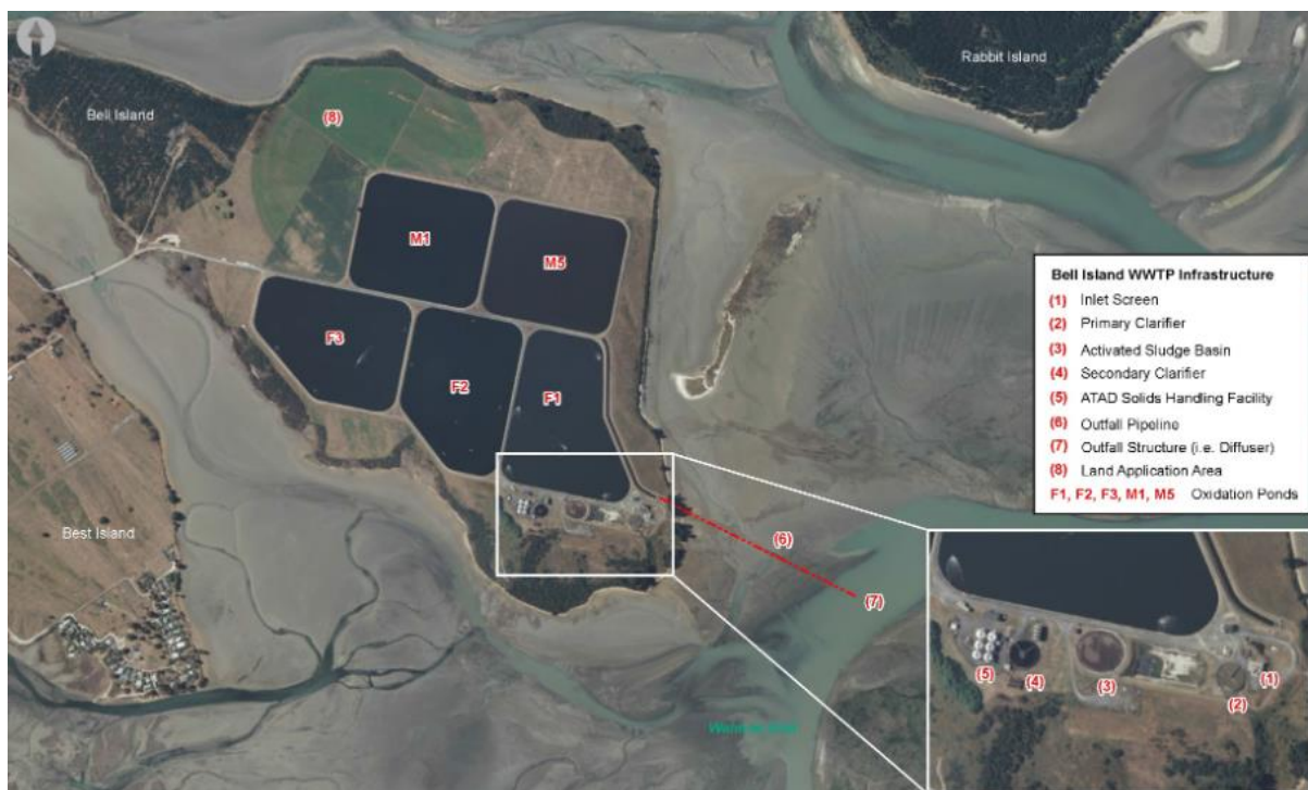
Figure 8-1: Main components of the WWTP (from Bell Island WWTP Application and AEE 2017)
