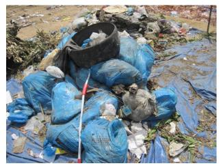
Figure 3-5 Sample placed on plastic sheet to allows fines to be collected
