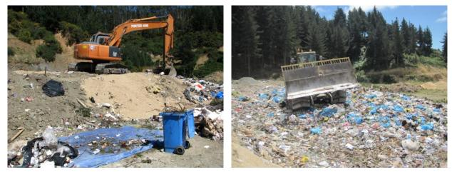
Figure 3-4: Excavator and compactor used at York Valley Landfill
